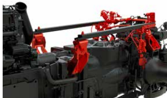
The semi-active, hydraulic cab suspension reliably absorbs jolting and vibrations.
